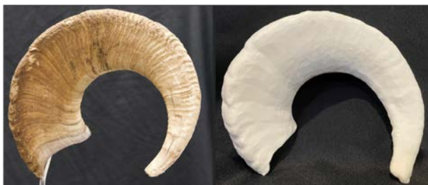
Figure 5. Visual comparison of a photograph of a horn from a deceased eight and half year-old ram to the 3D printed model of the horn. Note the visibility of the annuli, breakage, and shape. Model and photo by T.C. Henry.
